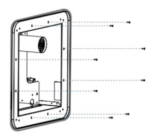
6. Apply sealant (**not included**) evenly around the door frame to fill any gaps with the RV's wall, then wipe off any excess sealant.
