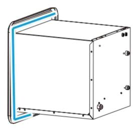
3. Insert the water heater into the opening, ensuring the butyl tape completes a tight seal between the RV siding and the door frame.
